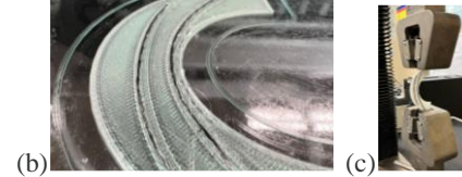
Figure 9: (a) Working Principle of the 3D Printer, (b) Fiber Path Detail, and (c) The MTS Sintech 10/D Fixture with the Half Loop
